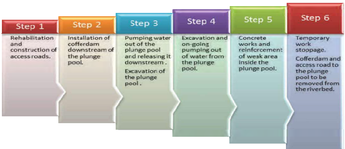
Figure 1.8 Sequencing of plunge pool construction activities
