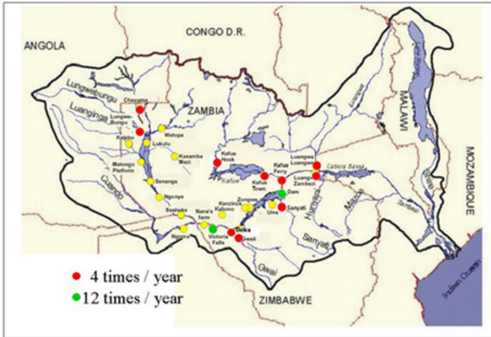
Figure 12. Location of the Authority’s Water Quality Sampling Sites in the Zambezi Basin
